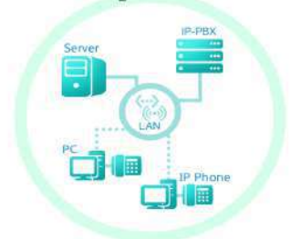
A company office using an IP-PBX
